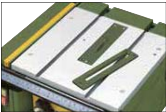
Non-slotted sawing cap cover of ABS for tight tolerances between saw blade and table (is slotted from below by the FET saw blade). For cutting very small parts.
